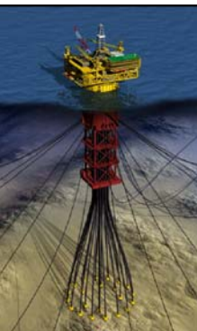
J P Kenny has engineered risers and subsea tie-backs for Spar systems such as Mad Dog.
