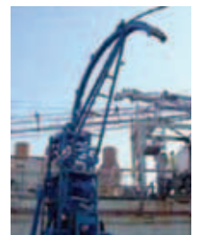
Deploying Coiled Tubing.
